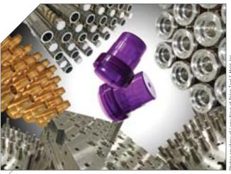
Pelco builds high-cavity stack tools utilizing copper alloys.
